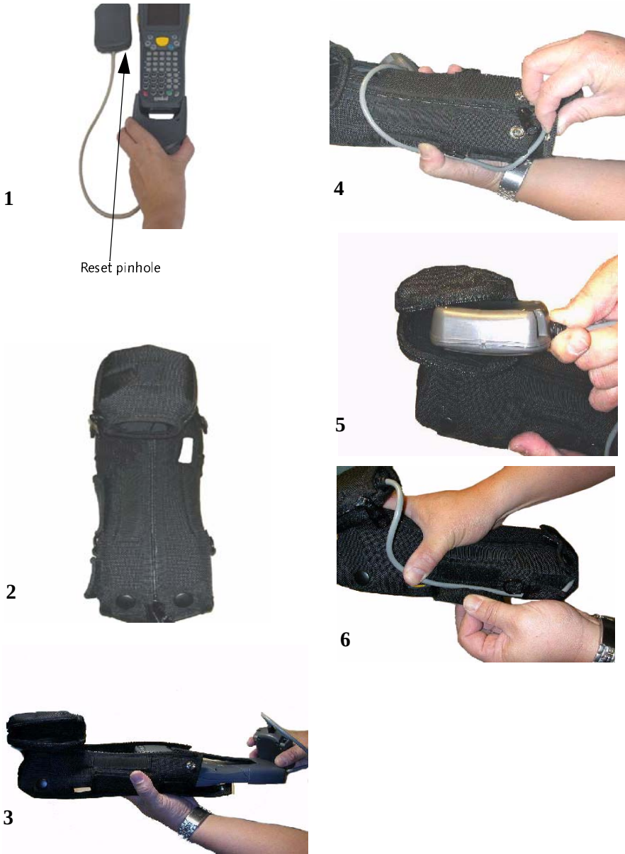
Figure 4 SMR-650P Pod Connection and Carrying Case Usage
