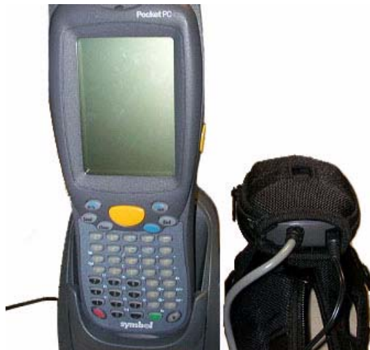
Figure 6 Charging the Handheld in the Carrying Case
