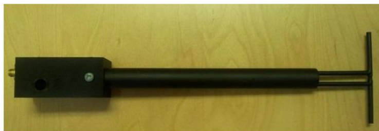
Figure 1 – MVG COMOSAR Validation Dipole
