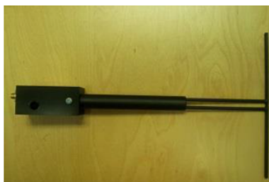
Figure 1 – MVG COMOSAR Validation Dipole
