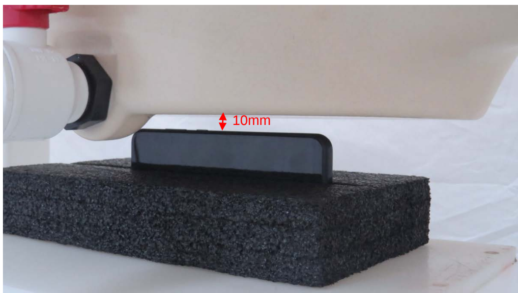
Picture 14: Right Side, the distance from handset to the bottom of the Phantom is 10mm
