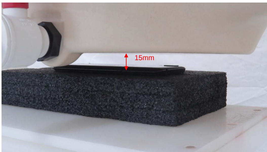
Picture 7: Back Side, the distance from handset to the bottom of the Phantom is 15mm
