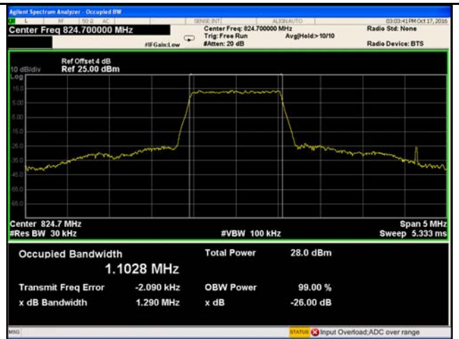
LTE Band V - Low CH 16QAM-1.4
