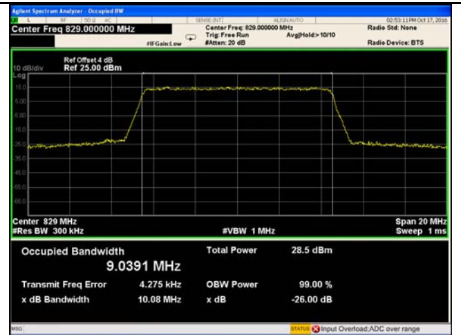
LTE Band V - Low CH 16QAM-10
