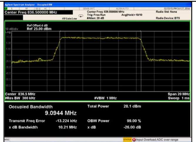
LTE Band V - Middle CH 16QAM-10
