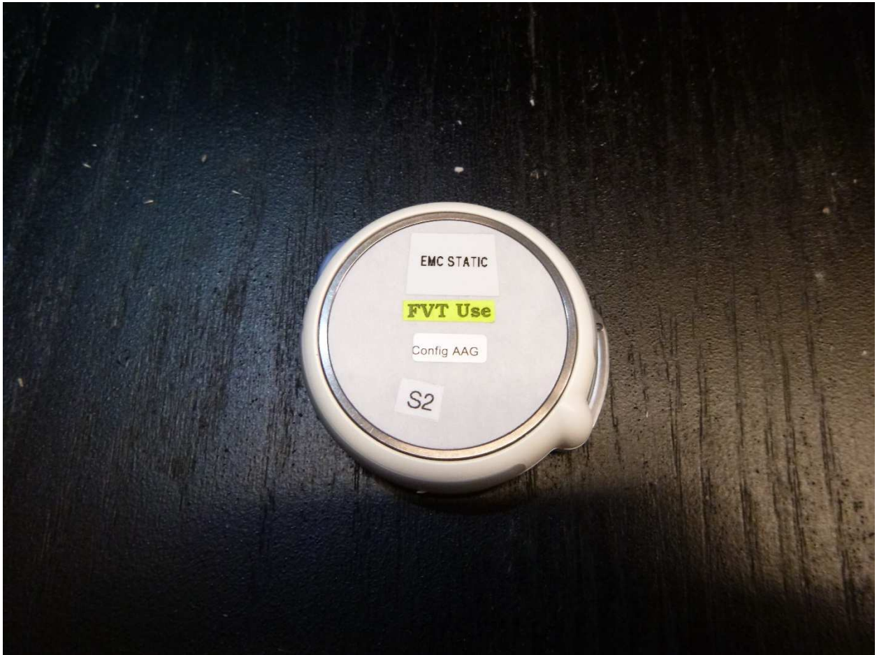
Front of Enclosure
