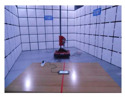
Photo of Setup for Radiated Emission (Bellow 1 GHz)
