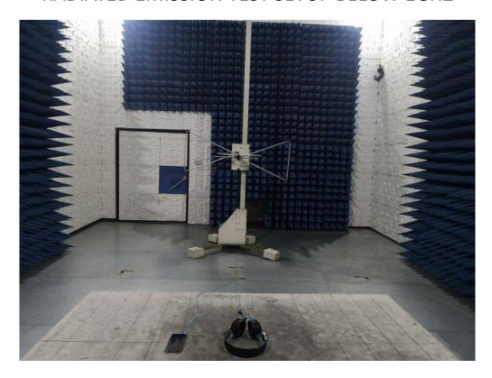
RADIATED EMISSION TEST SETUP ABOVE 1GHZ
