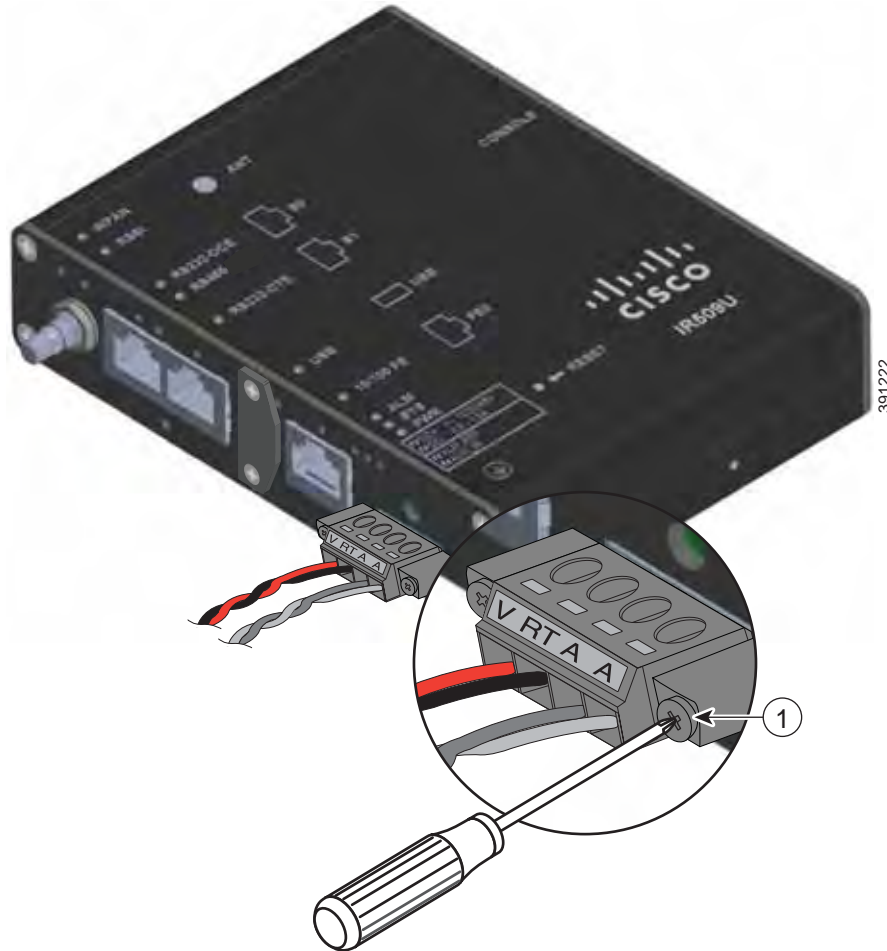
Figure 2-23 Connecting the Power and Alarm Connector to the WPAN Gateway
