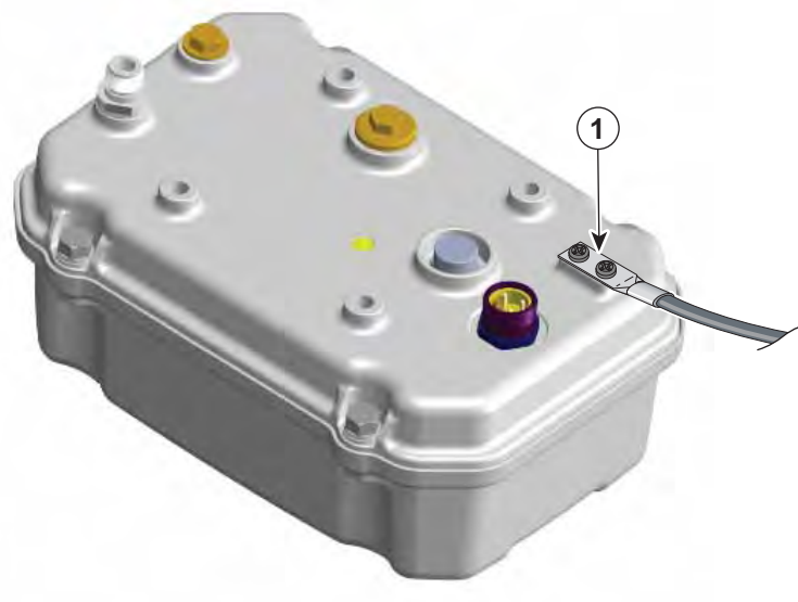
Figure 2-18 Installing the Ground Lug
