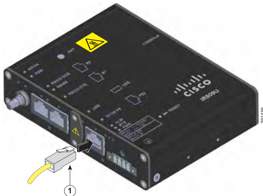
Figure 2-25 Connecting to the 10/100 Fast Ethernet Port
