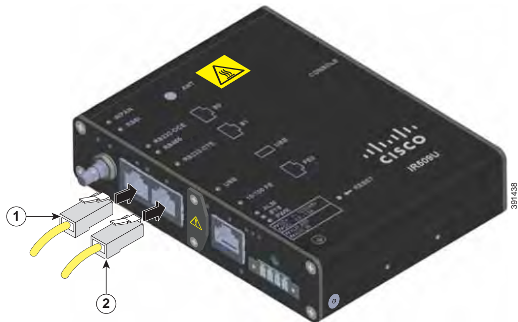
Figure 2-24 Connecting to the RS232DCE/RS485 or RS232-DTE Ports
