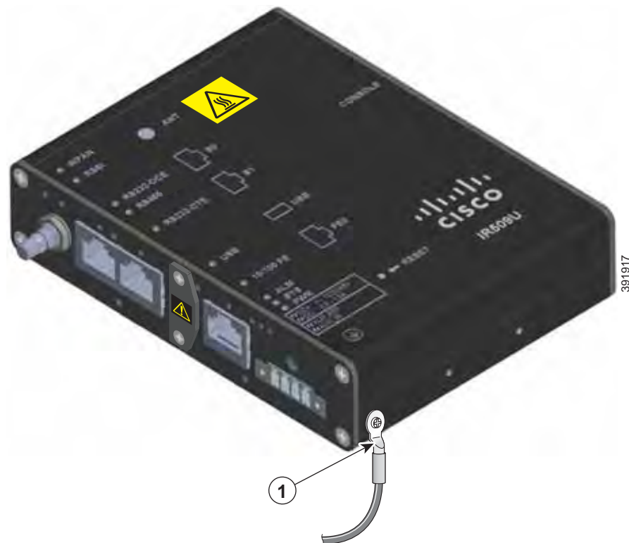
Figure 2-10 Installing the Ground-Lug Screw
