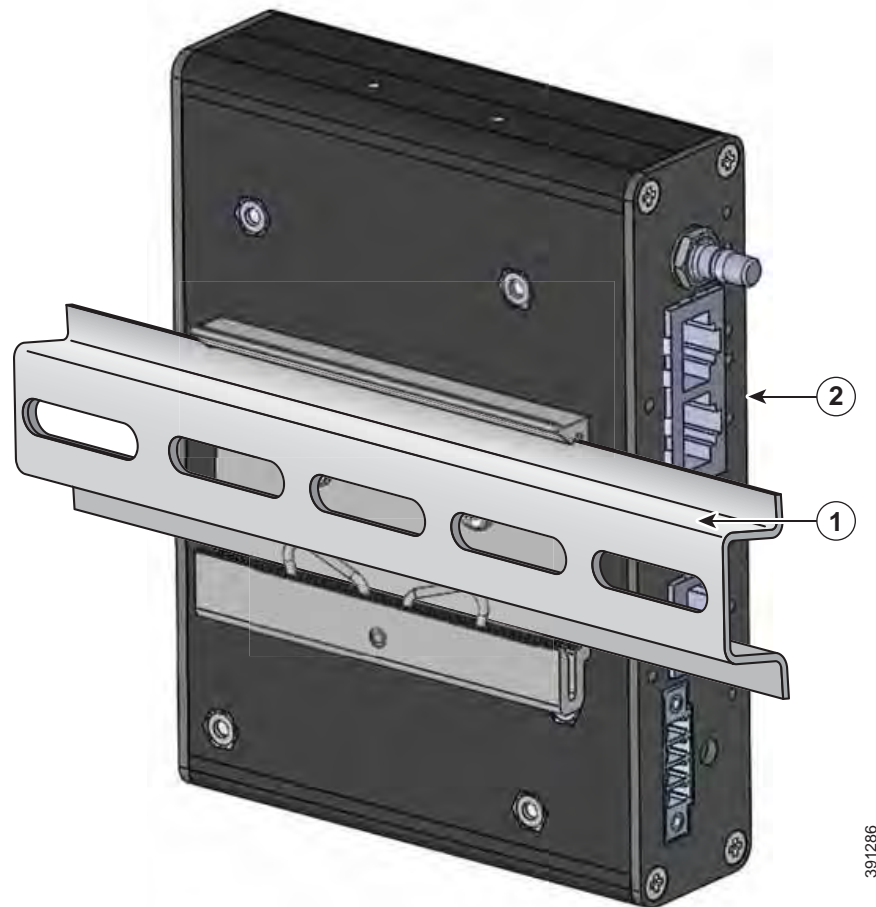
Figure 2-4 WPAN Gateway Mounted on the DIN Rail
