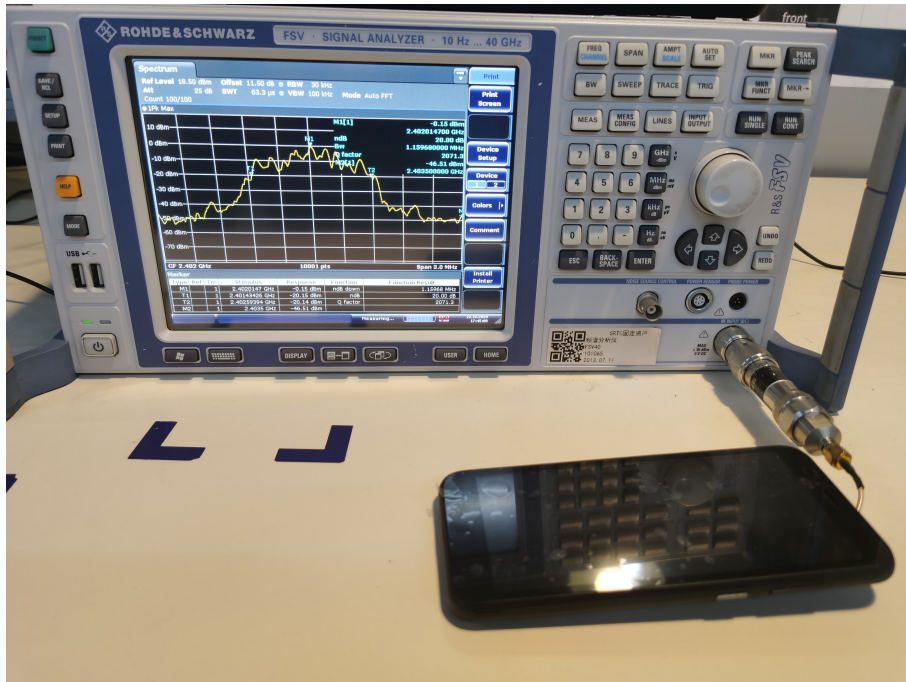
RF Conducted Test setup (BT/BLE/WIFI)
