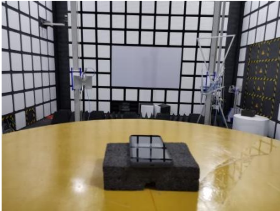
Spurious Radiated Emissions Test setup
