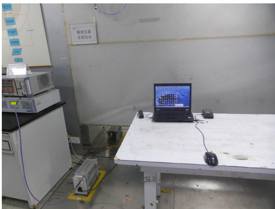
Conducted Emissions Test Setup
