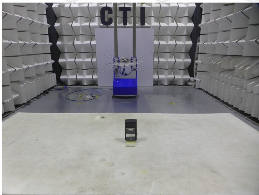
Radiated spurious emission Test Setup-2(30MHz-1GHz)
