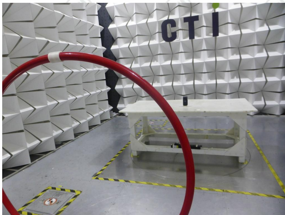
Radiated spurious emission Test Setup-1(9kHz-30MHz)
