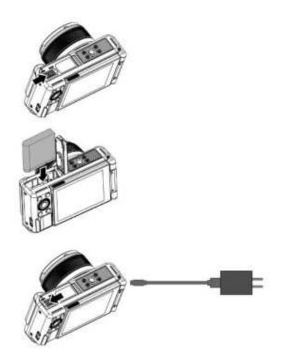
•Install the battery into the camera according to the direction shown in the diagram.
