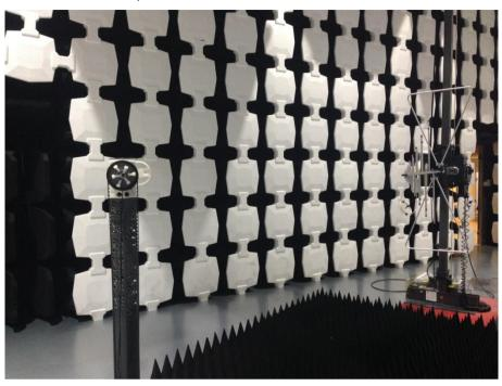
Description: Substitution Antenna for ERP Test
