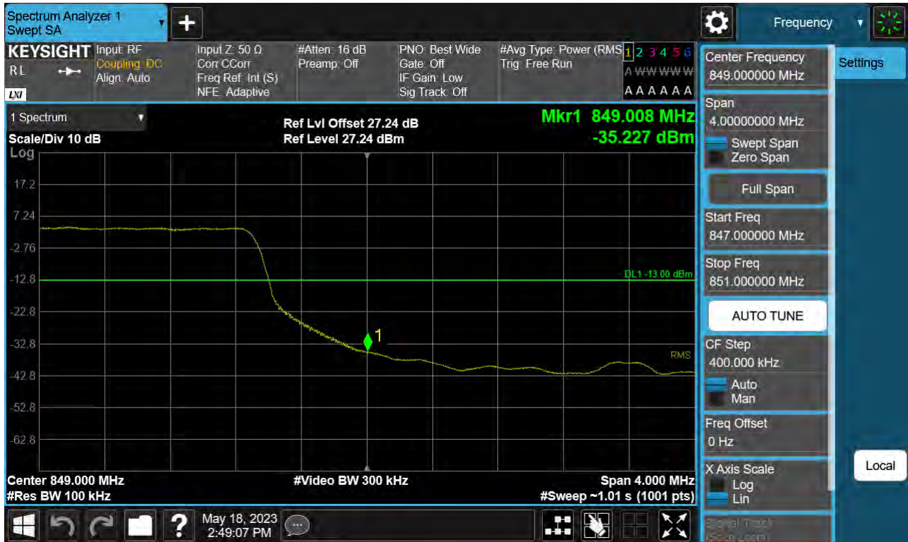
Sub6 n5. Upper Band Edge Plot (10 M BW Ch.168800 BPSK_RB50_Offset 0)
