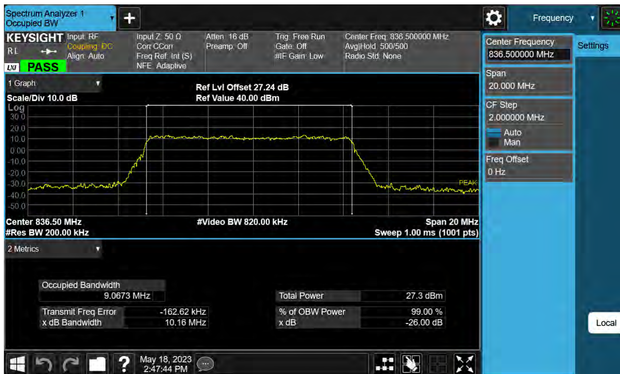
Sub6 n5. Occupied Bandwidth Plot (10 M BW Ch.167300 256QAM_ Full RB _0)
