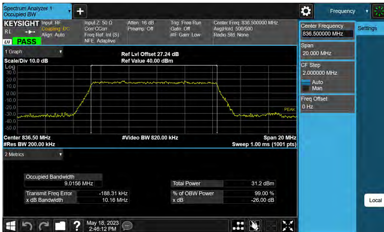
Sub6 n5. Occupied Bandwidth Plot (10 M BW Ch.167300 BPSK_ Full RB _0)
