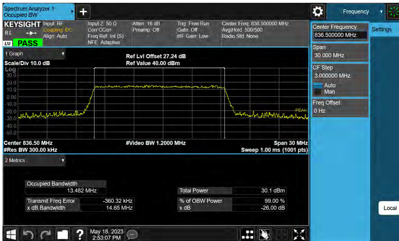
Sub6 n5. Occupied Bandwidth Plot (15 M BW Ch.167300 16QAM_ Full RB _0)
