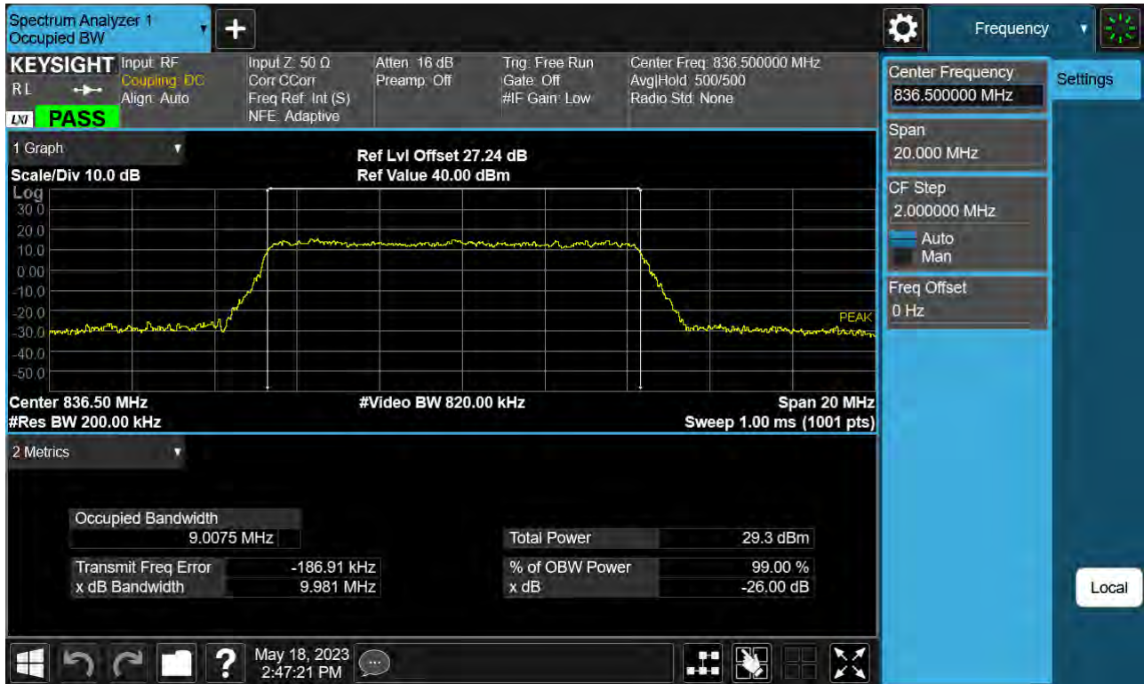
Sub6 n5. Occupied Bandwidth Plot (10 M BW Ch.167300 64QAM_ Full RB _0)
