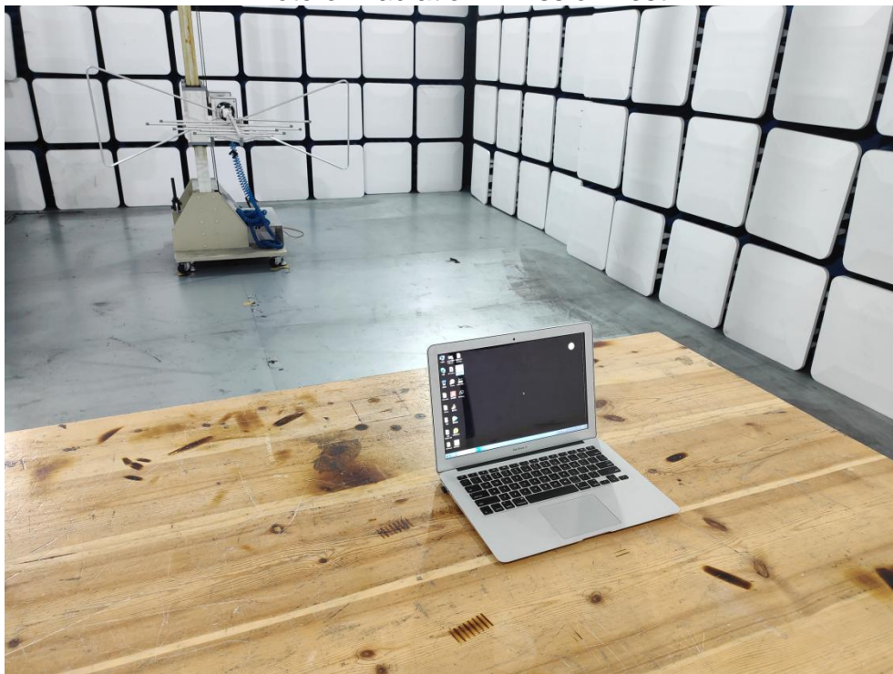
Photo of Radiation Emission Test
