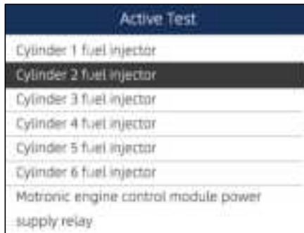
Figure 5-25 Sample Active Tests Selection Screen
