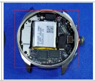
The antenna is Metal frame antenna.
