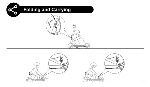
Make sure that the scooter's turned off. To fold, unlock the folding mechanism, and bend the handlebar stem to hook the buckle on the rear fender. To open, press the bell trigger to remove from the buckle, erect the handlebar and lock the folding structure.
