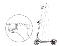
3. When the scooter starts to coast, put both feet on the deck and press the accelerator (the accelerator initiates once the coasting speed exceeds 3mph)
