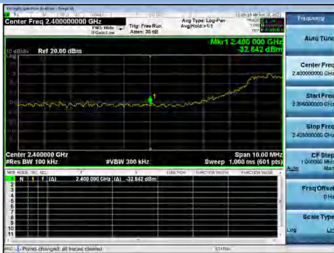
802.11n-40 MHz LOW CHANNEL, Carrier level
