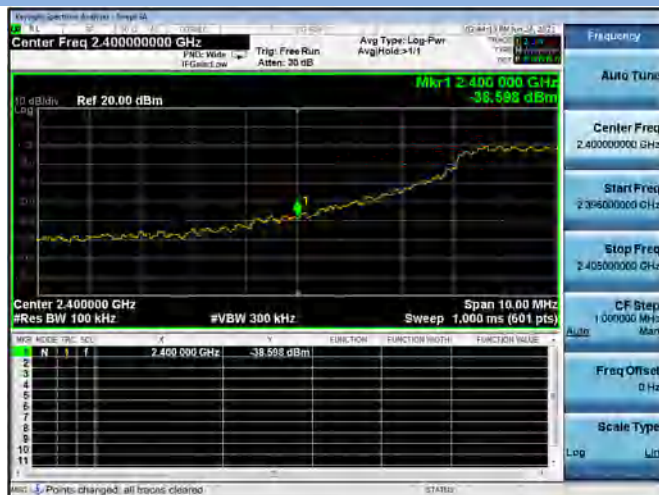
802.11n-20 MHz LOW CHANNEL, Carrier level
