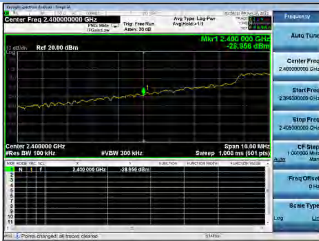
802.11n-40 MHz LOW CHANNEL, Carrier level
