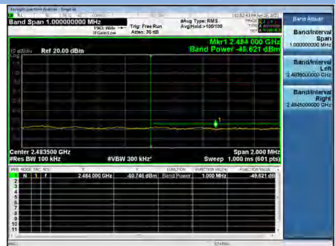
802.11n-20 MHz HIGH CHANNEL, Reference level
