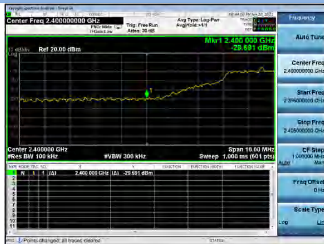
802.11n-20 MHz LOW CHANNEL, Carrier level
