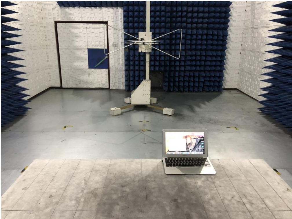
FCC RADIATED EMISSION TEST SETUP ABOVE 1GHZ
