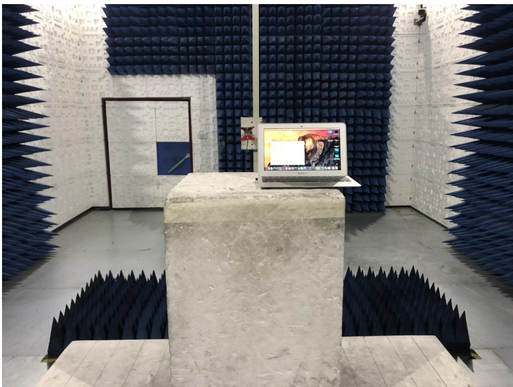
FCC RADIATED EMISSION TEST SETUP ABOVE 1GHZ
