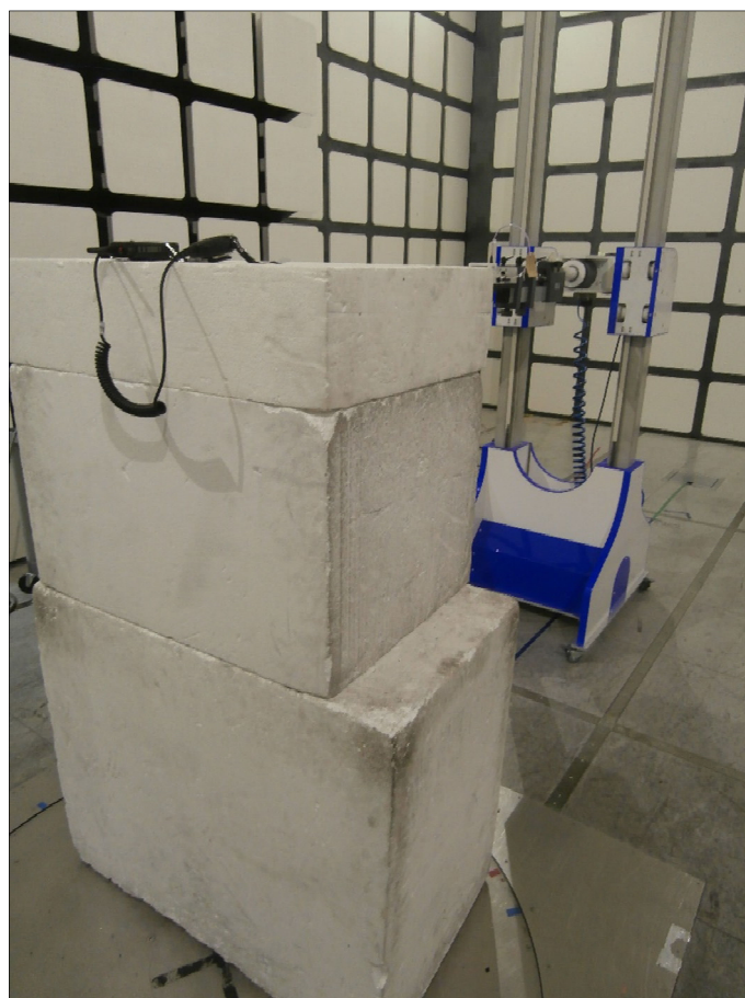
Figure 148 - Test Setup - 18 GHz to 25 GHz
