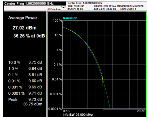
Channel: MIDDLE, Modulation: 64QAM, BW=15MHz, CCDF
