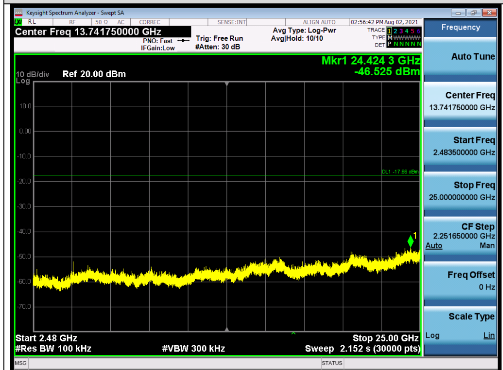
Test_Graph_802.11b_ANT1_2412_1Mbps_Higher Band Emissions
