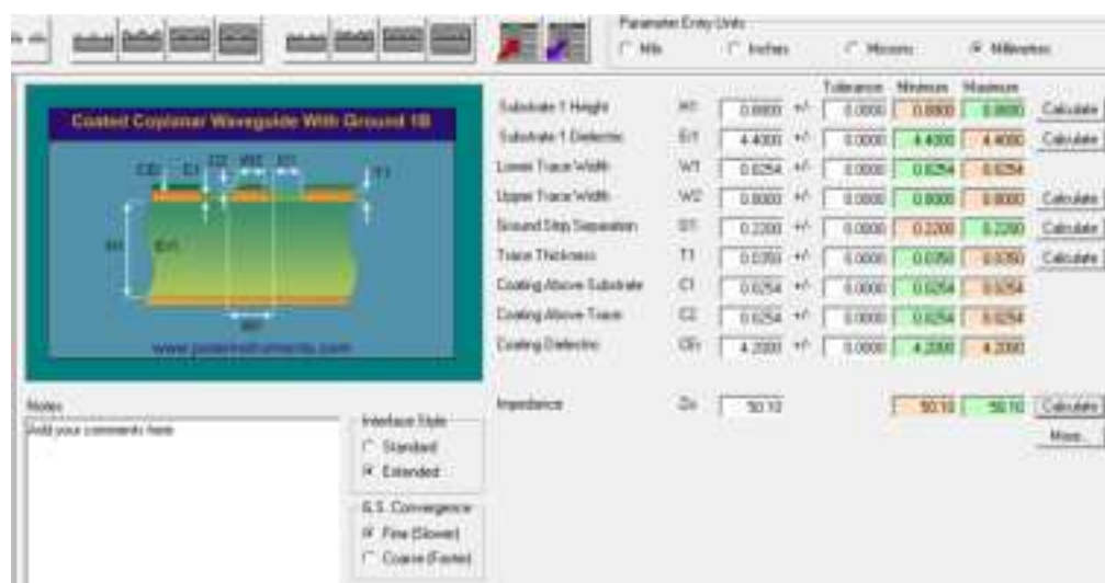
Figure 7. SI9000 Impedance Calculation Diagram
