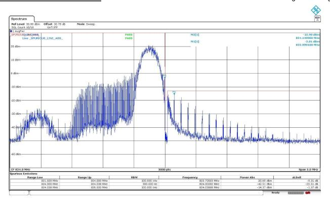
Sub-band 814-824 MHz. EA MASK: BW=1.4 MHz. RB Size=5. RB Offset=1. Narrow Band=0. High Block Edge:
