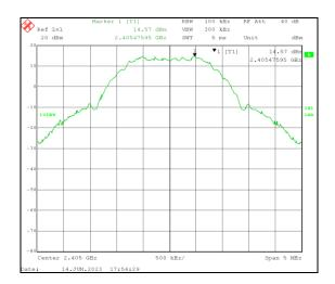
The peak level of 14.6 dBm is the maximum peak output of the Lutron Model JPZ0148 LED Lighting Controller. The conducted spurious emissions from the antenna port must be 20 dB down from this peak. The resultant limit is therefore -5.4 dBm and is displayed on the plots below.
