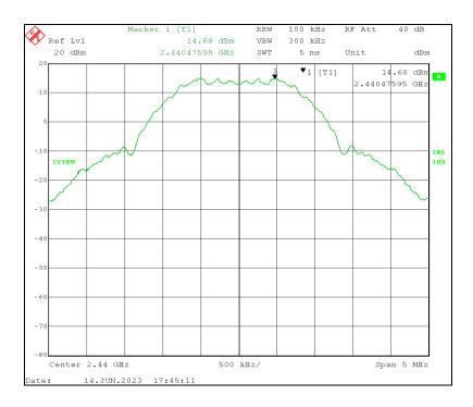
The peak level of 14.7 dBm is the maximum peak output of the Lutron Model JPZ0148 LED Lighting Controller. The conducted spurious emissions from the antenna port must be 20 dB down from this peak. The resultant limit is therefore -5.3 dBm and is displayed on the plots below.
