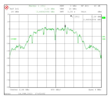
BEC-2259-01A REV2 Lutron JPZ0148 802.15.4 Radio FCC Part 15.247 DTS Test Report Release Date: 08/28/2023 Page 45 of 65
