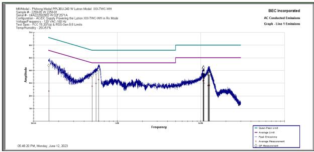
**Results:** The Lutron Model JPZ0148 Sample 2259-01 powered by the Lutron Electronics Model T120-24DC-15 Sample 2259-05 complies with the requirements of FCC Part 15.207. The margin is 2.79 dB @ 9.247 MHz with Sample 2259-01 transmitting Low Channel, 2405 MHz, Phase Line.
