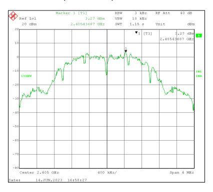
Channel 18, 2440.0 MHz, O-QPSK Modulation
