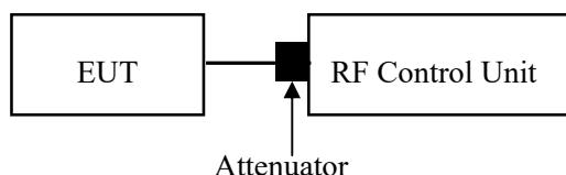
Note: the RF control unit has a built-in power sensor.
