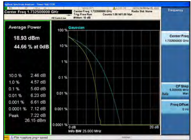
Band4 / 15MHz / Mid CH / 64QAM
