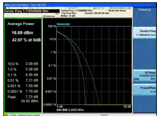
Band66 / 3MHz / High CH / 64QAM
