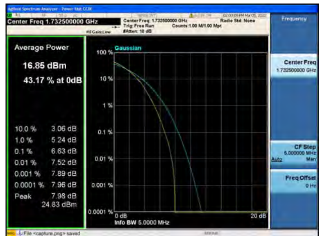
Band4 / 5MHz / Mid CH / 64QAM
