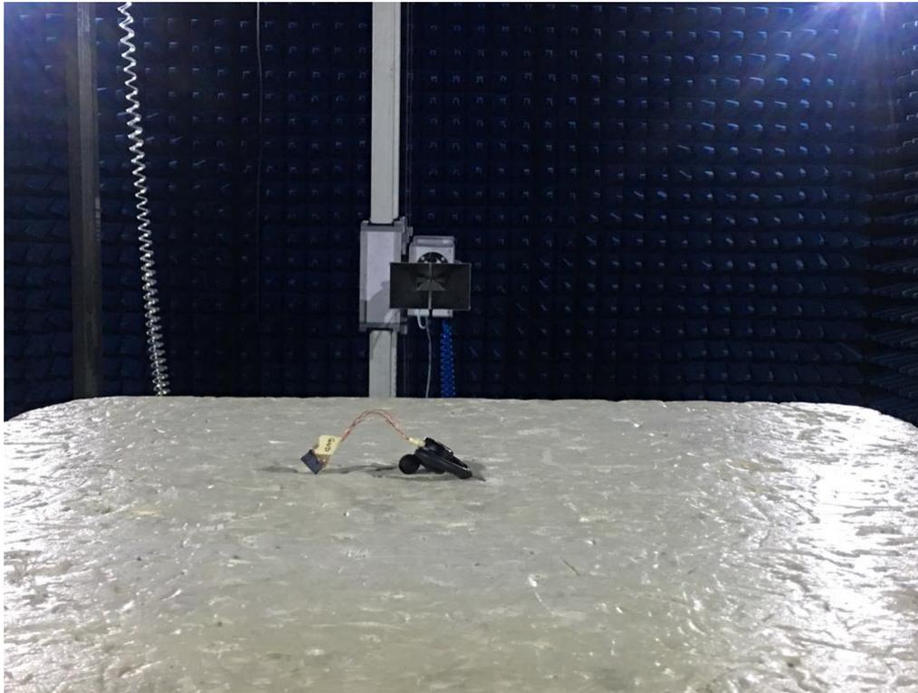
**Photograph 2: Set-up for Spurious Emissions (18GHz-26GHz)**
