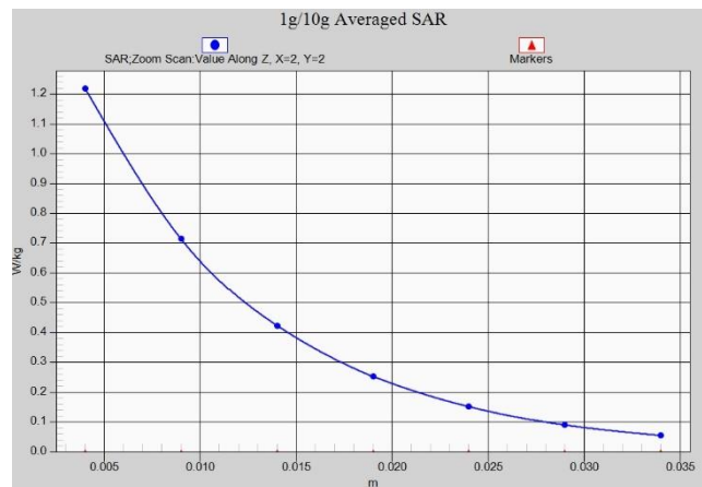
Fig. 1-18 Z-Scan at power reference point (LTE Band25)
