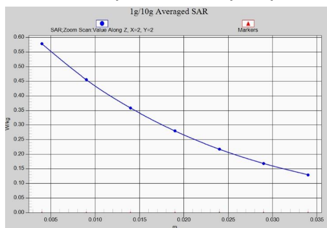
Fig. 1-14 Z-Scan at power reference point (LTE Band 12)
