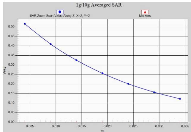
Fig. 1-16 Z-Scan at power reference point (LTE Band13)
