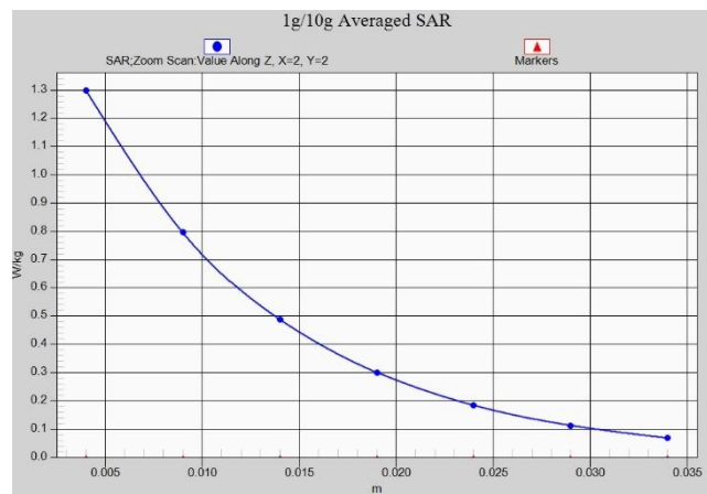
Fig. 1-28 Z-Scan at power reference point (LTE Band66)
