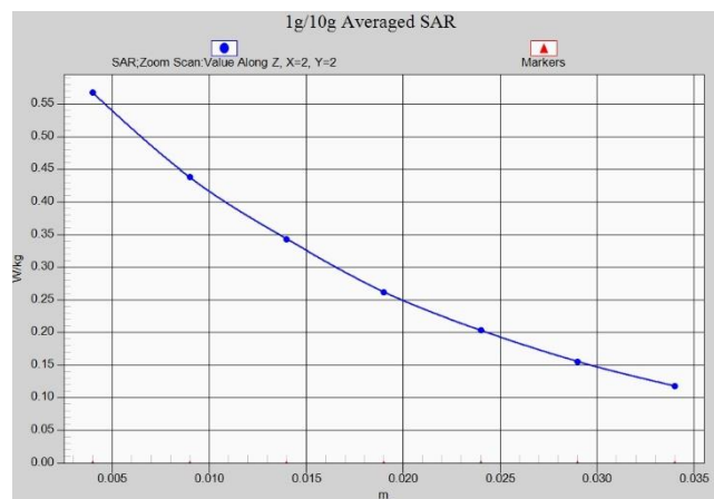
Fig. 1-12 Z-Scan at power reference point (WCDMA850)
