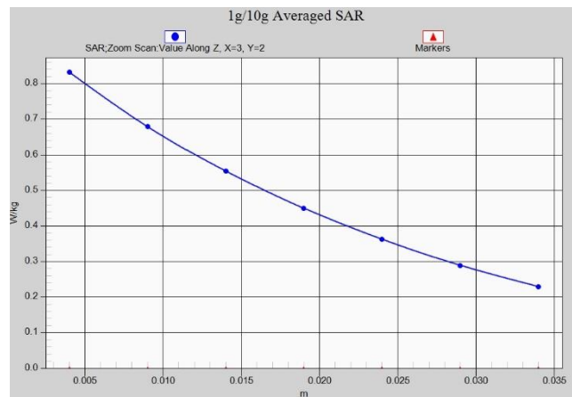
Fig. 1-21 Z-Scan at power reference point (LTE Band26)
