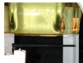
Fig. 9 Body SAR Test Setup
