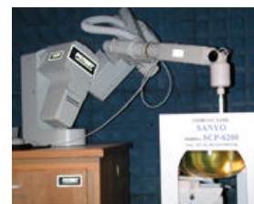
Fig. 1 SAR Test Setup
