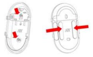
3. Attach the device to the mount bracket.
