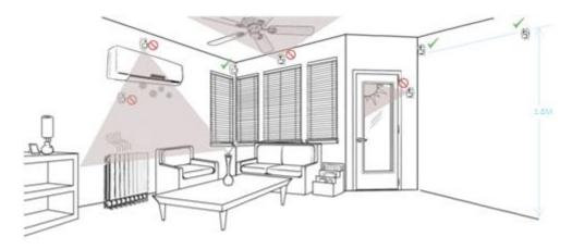
The recommended mounted position for a Motion Sensor should be 1.8M from the floor in the corner of a room. At this height, the device can detect a movement up to  $10M \, (\pm 1M)$  (see the following image). Also, in this position, the 90 degrees ( $\pm 10 \, \text{degree}$ ) fanshaped detection pattern can normally offer greater protection than mounting on a flat wall.
