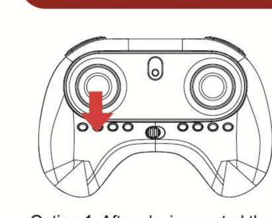
Option 1: After playing, control the drone to the ground and keep the throttle at the lowest position for 3-4 seconds or until the motor stops working. Finally switch off the transmitter and drone.
