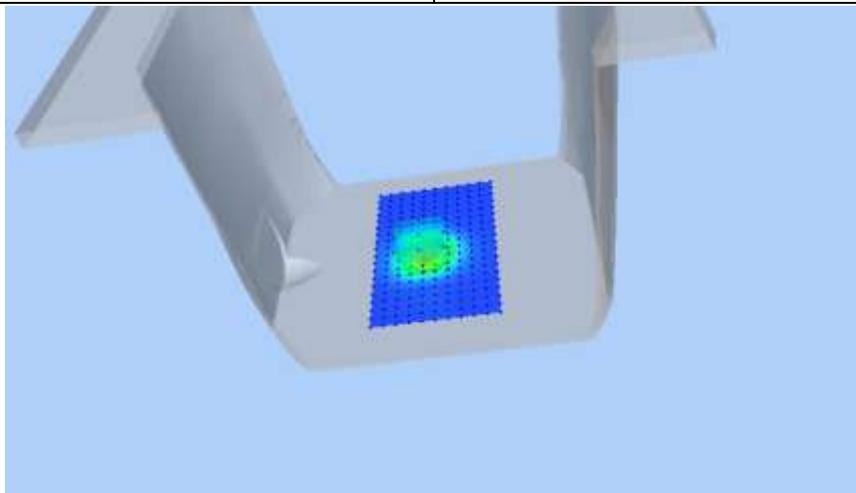
Test Mode:802.11A,MID channel(Body SAR-LCD DOWN)
