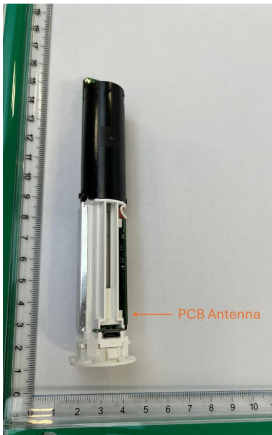
Figure 5: PCBA mounted on the back of the chassis.
