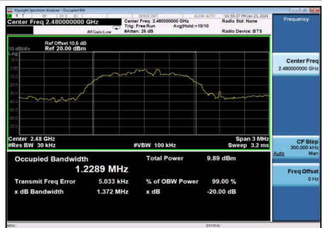
20dB Bandwidth: DQPSK,2480MHz,2DH5
