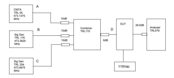
The Intermodualation and spurious products were measured with the amplifier operating at maximum gain. A three tone test was conducted using the equipment as above. The input power level was adjusted so the level at point D was the maximum input of –29.1dBm The cable and attenuator loss between the EUT and the spectrum analyser was 26.6dB.
