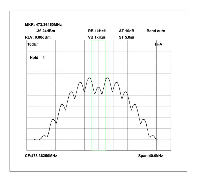
473.3625MHz Signal Generator deviation set to 5kHz
