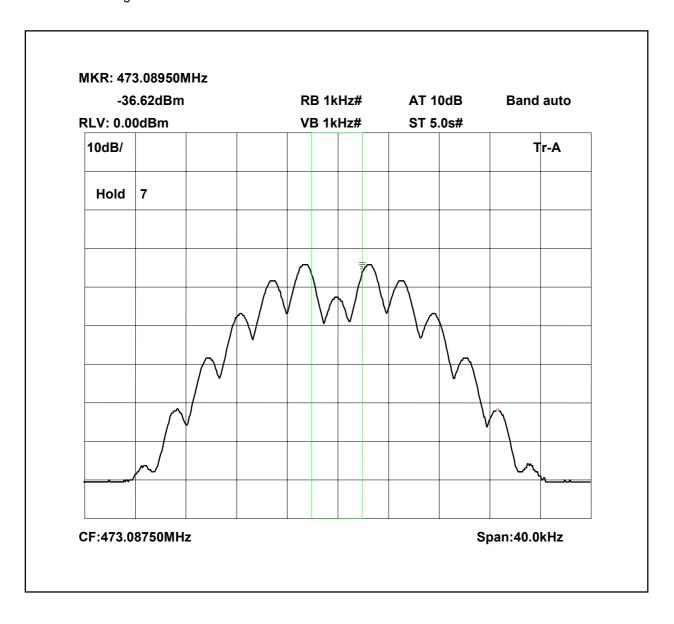
473.0875MHz Signal Generator and EUT deviation set to 5kHz
