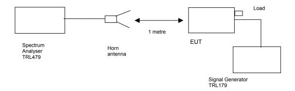
The test was set up as per the diagram. The level at the input was adjusted to compensate for the loss of the interconnecting cable. The unit was tested operating maximum power on three test frequencies with a 50 ohm load on the output. The unit was also tested with the signal generator replaced by another 50ohm load.
