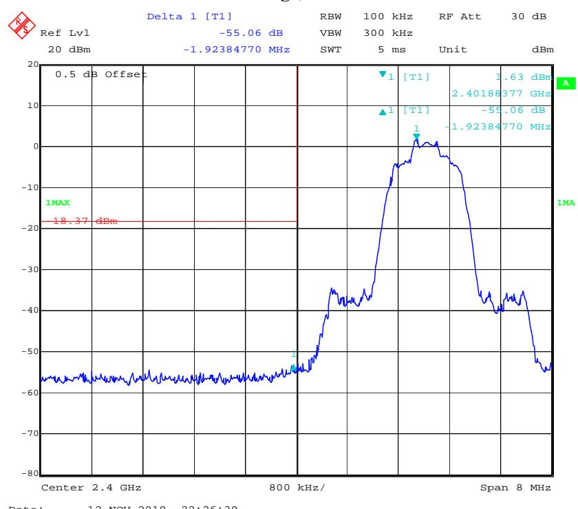
**Band Edge, Right Side**
