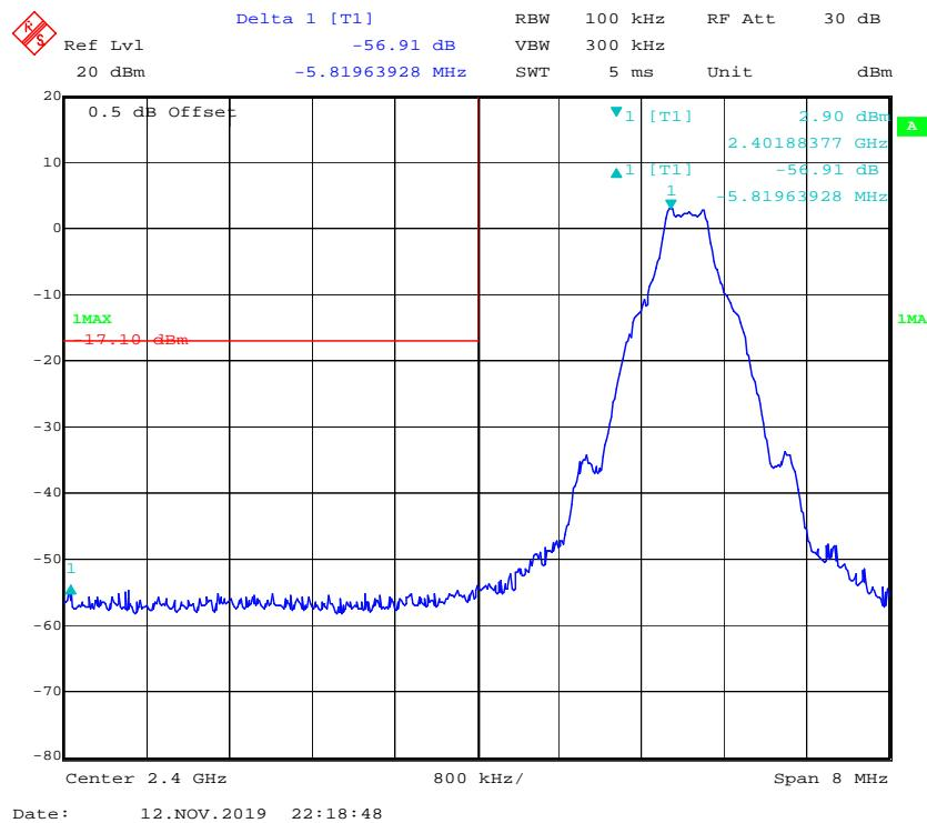
**Band Edge, Right Side**
