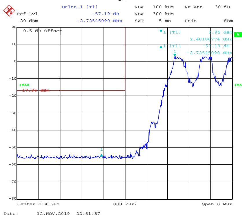
**Band Edge, Right Side**
