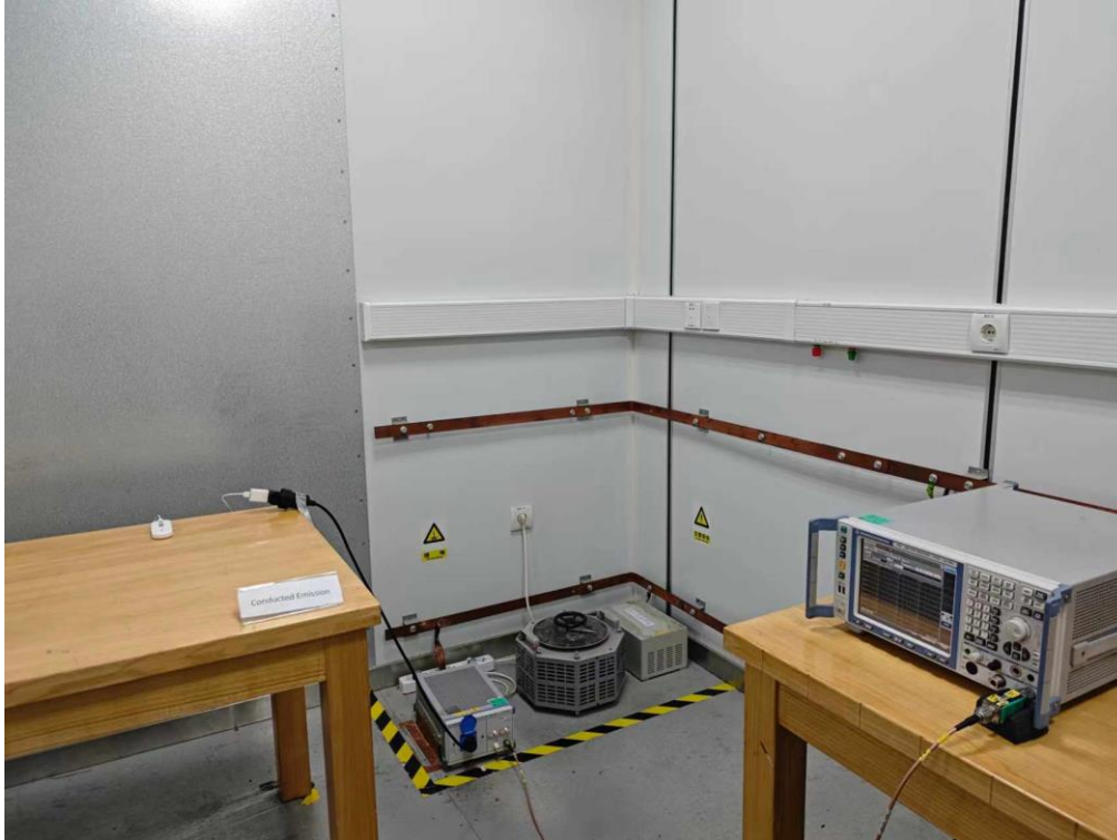
Radiated Emission Setup 9kHz-30MHz
