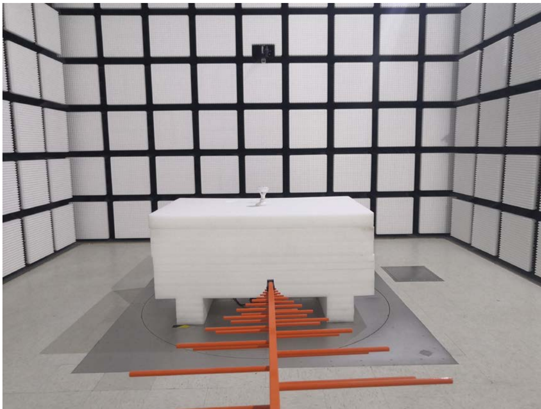
Radiated Emission Above 1GHz View
