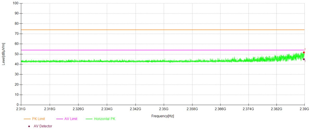
Test Model **Spurious Emission in Restricted Band 2310-2390MHz**
