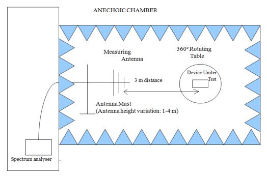
$Shielded\,Control\,RoomFor$ Radiated Measurements
