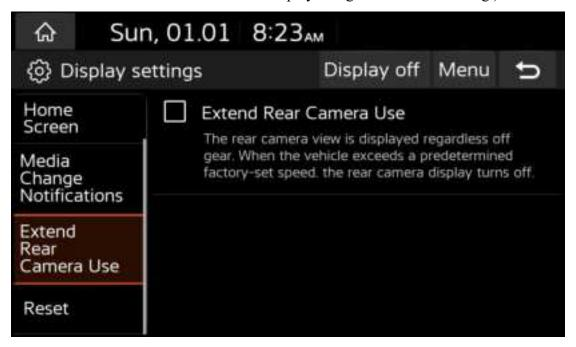
When the vehicle speed exceeds the preset factory set speed, the rear camera is off.
