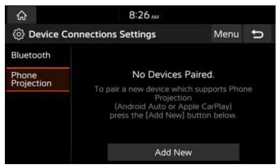
Click [add new] to search for available wireless carplay devices. Press the cancel button to stop the search. You can pair up to 8 devices. Click the Connect button to connect to the paired device, and click the Delete button to delete the paired device.
