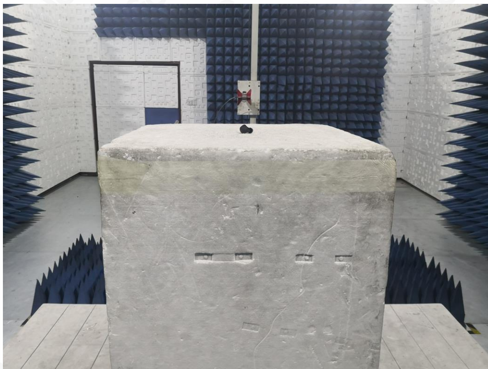
RADIATED EMISSION TEST SETUP ABOVE 1GHZ
