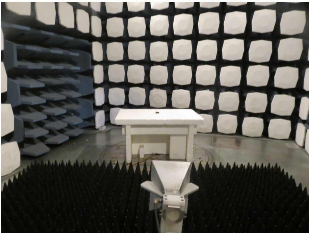
Radiated Spurious Emissions Test setup
