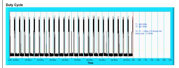
**NOTE:** T1 denotes the start of duty cycle period is  $0^{th}$  second. T2 denotes the end of duty cycle period is  $1^{th}$  second. T2 – T1= 1 seconds. Duty Cycle = 17.393%
