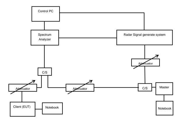
The EUT is a U-NII Device operating in Client mode without radar detection. The radar test signals are injected into the Master Device.
