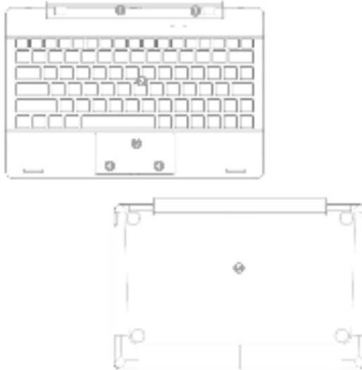
1.- Movable base keyboard interface: This interface is magnetic, which is convenient for alignment and firmly linking the Table PC and the keyboard.
