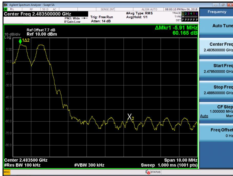
Test Plots with hopping (8DPSK)
