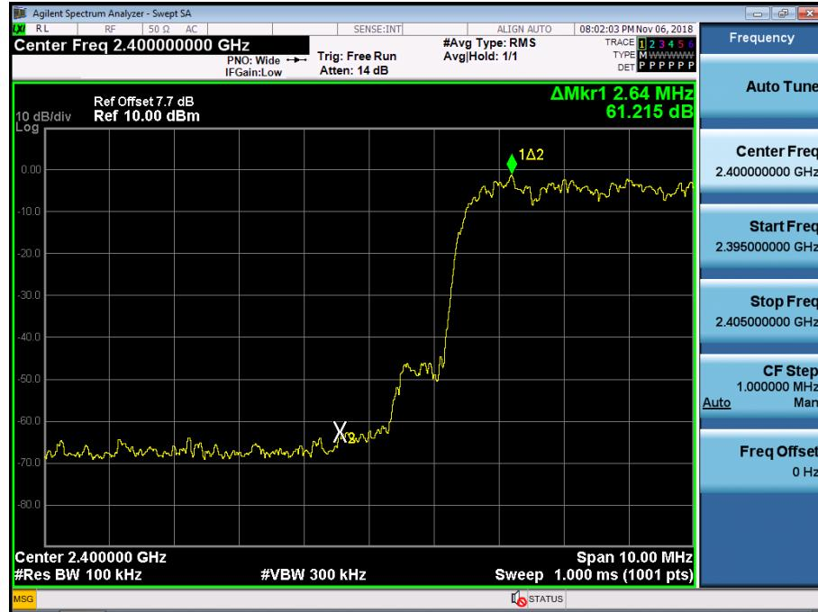
Test Plots with hopping (8DPSK)
