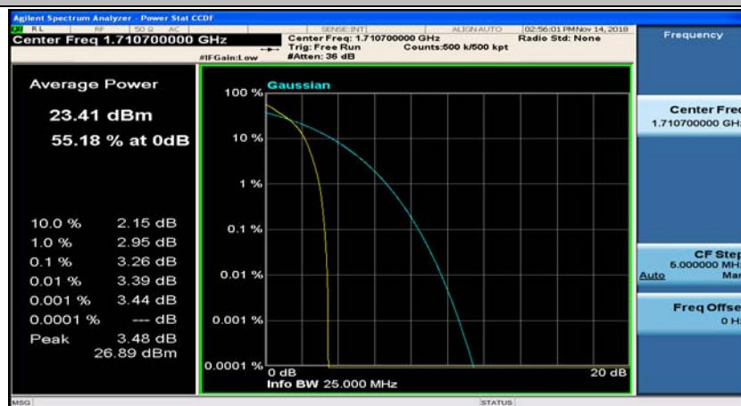
(Channel Bandwidth: 1.4 MHz)_LCH_QPSK_3RB#0
