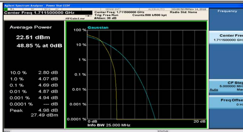
(Channel Bandwidth: 3 MHz)_LCH_16QAM_8RB#0
