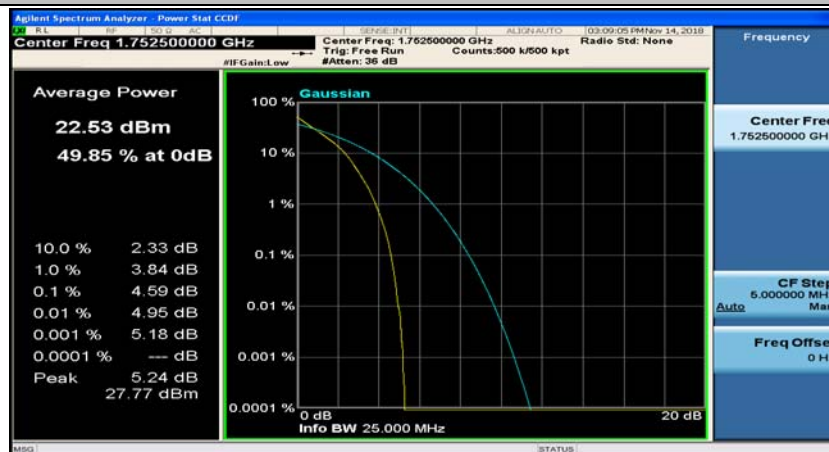
(Channel Bandwidth: 5 MHz)_HCH_QPSK_25RB#0
