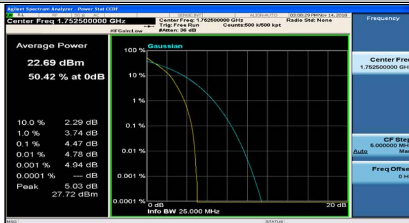
(Channel Bandwidth: 5 MHz)_HCH_QPSK_12RB#6
