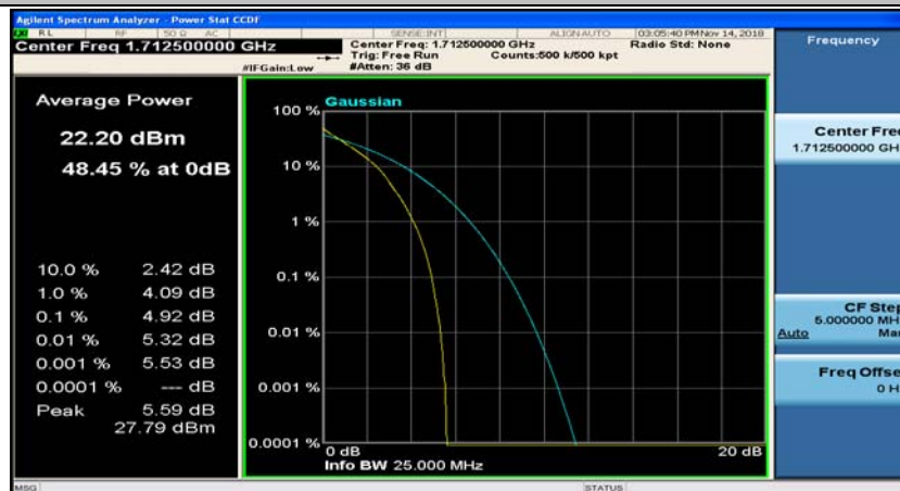
(Channel Bandwidth: 5 MHz)_LCH_QPSK_25RB#0
