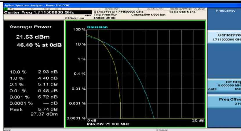
(Channel Bandwidth: 3 MHz)_LCH_16QAM_15RB#0
