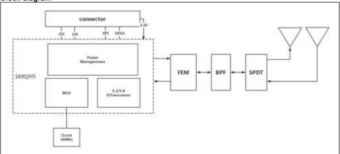
Note: Frequencies of this transmitter 5160-5245MHz & 5730-5845MHz.
