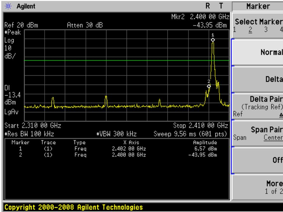
GFSK mode: Band Edge-High Channel
